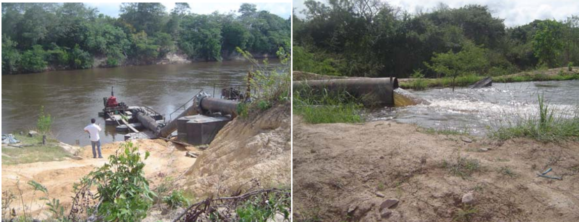
Figures 13 and 14: Pumping Water from the Ireng River to Irrigate Rice
